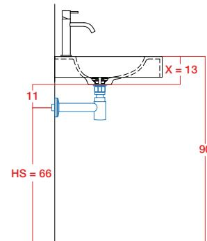
$$\begin{aligned} \text{HS} &= 90 - (X + 11) \\ (X + 11) &= 13 + 11 = 24 \text{ cm} \\ \text{HS} &= 90 - 24 = 66 \text{ cm} \end{aligned}$$
